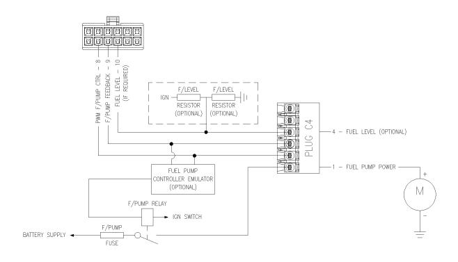
FUEL SYSTEM WIRING (VARIABLE EMULATED)
