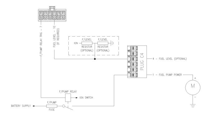
FUEL SYSTEM WIRING (NON VARIABLE)
