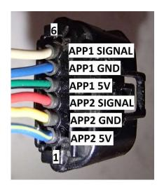
**Late Model Pedal Plug Wiring**
