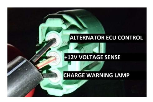
Typical late model Alternator plug (with all 3 connections)
