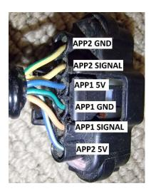
**Early Model Pedal Plug Wiring**
