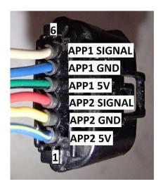
**Late Model Pedal Plug Wiring**
