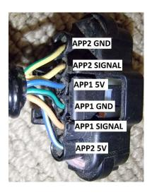
**Early Model Pedal Plug Wiring**
